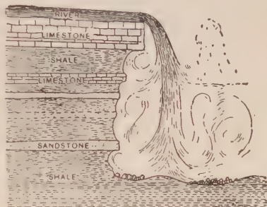
FIG. 66. — An ideal section of Niagara Falls, showing how the soft shales are being worn away, leaving the limestone above unsupported. (Gilbert.)
